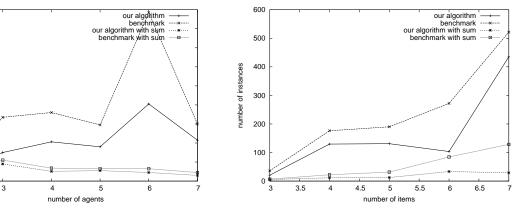
(c) Number of instances before failure in localVCG: Agents. (d) Number of instances before failure in localVCG: Items.
